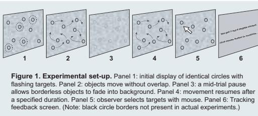
**Figure 1. Experimental set-up.** Panel 1: initial display of identical circles with flashing targets. Panel 2: objects move without overlap. Panel 3: a mid-trial pause allows borderless objects to fade into background. Panel 4: movement resumes after a specified duration. Panel 5: observer selects targets with mouse. Panel 6: Tracking feedback screen. (Note: black circle borders not present in actual experiments.)
